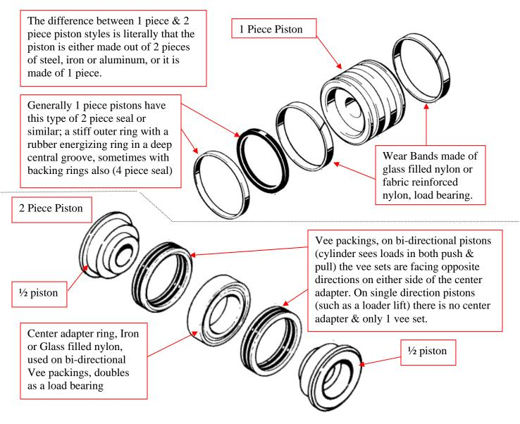
This is just a typical example & your cylinder construction may vary greatly, however the terminology is generally applicable to a wide variety of designs. Please note that when  $\underline{we}$  refer to the  $\underline{piston}$  we are referring to the part of the cylinder called the piston, not the entire hydraulic cylinder.
