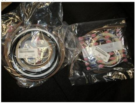
include metal backed rod bearings (Pictured below left), the only general exception is John Deere excavators. Kobelco kits (in picture above), and Komatsu do not include the metal backed rod bushings. Hitachi kits do not include the metal bushing or the piston wearbands & Teflon scraper rings (below), but the JD kits are all inclusive for the same equipment (JD excavators are Hitachi's with a JD engine). These items are usually
