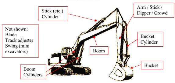
Cylinders are named for the part of the machine they move i.e. bucket &/or the type of movement they cause i.e. boom lift. Thumbs & twist-o-wrist cylinders are add on equipment & generally not listed as they could be mfg'd by many vendors. Many blade cylinder kits are available, but be aware that these kits are for OEM blades & will not fit add on aftermarket blades, even if it was installed by your dealer prior to delivery, it may still be an aftermarket add on blade & not original equipment.
